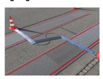
The purpose is to fix two sensors and four long levelling mats. It consists of two frames and one connecting plate.
