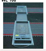
The purpose is to align two scales and four long levelling mats. It also facilitates shifting the scales laterally in order to adapt to the track width of the vehicle. The frame is equipped with a groove for the connecting cable.
