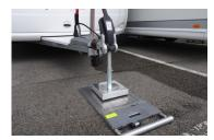
With the additional telescope support more applications are possible, such as weighing the down force of trailer couplings.
