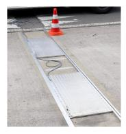
The mounting frame is used for lowering two scales into the pavement. In this case no levelling mats are required because the scale surface is flush to the pavement. This semi-permanent installation is advantageous if the weighing is always performed at the same location. The frame is equipped
