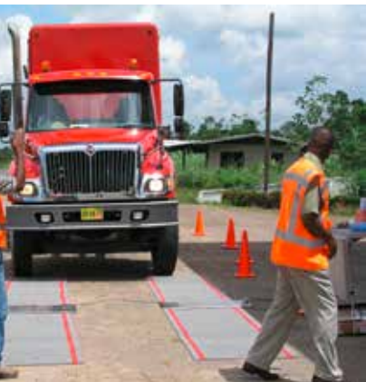
Pre-selection in Surinam with portable scales
