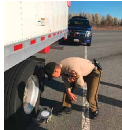
The mechanical scale WL 101 is widely used in the U.S. for the official weight enforcement
